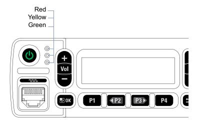
Blinking red – Radio is receiving an emergency transmission or has failed the self-test upon powering up, or has moved out of range if radio is configured with Auto-Range Transponder System.
